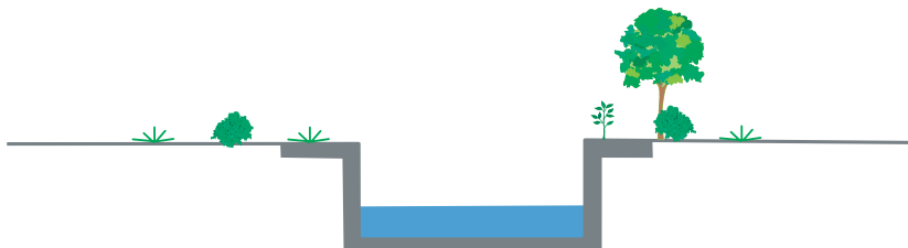
D. Concrete lined channel
